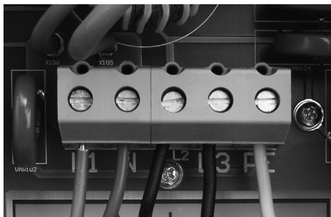
(Fig.) Circuit board terminal for fixing the grid cable
